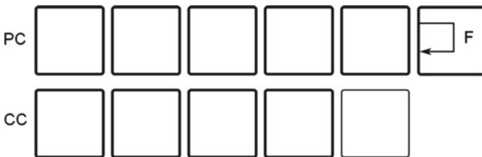
Fig. 29.29 Another example of edge detection in the matrix. A two-channel wire is grown to the right. At each step, a feedback cell (“F”) is configured; a test ping is sent; and an echo is detected. The echo detection will fail when the wire has reached the rightmost edge of the matrix (since there is no cell available for building the feedback cell). This allows a circuit to determine the horizontal width of the matrix. A similar technique can be used to determine the matrix’s height
