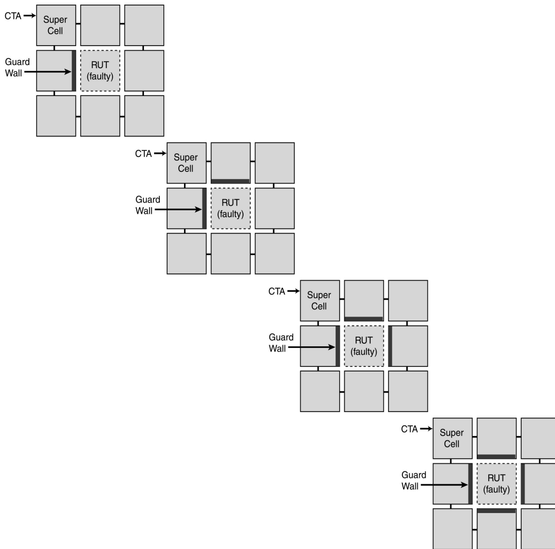
Figure 7. A 4-part time series showing the full activation of guard walls to isolate a faulty region. The faulty RUT is shown in the center.
